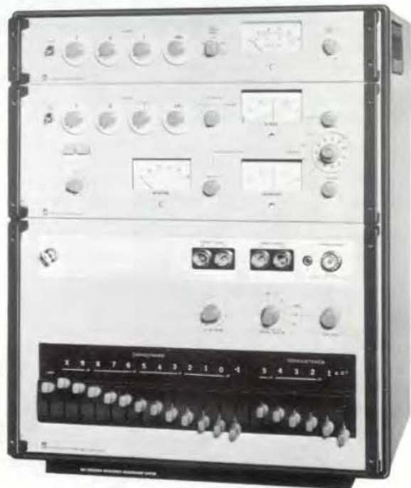
Figure 8. GR Precision Capacitance-Measurement System. Top to bottom: 1316 Oscillator, 1238 Detector, 1616 Precision Capacitance Bridge
